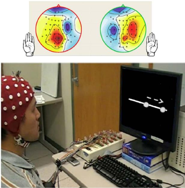
**Fig. 6.** An example EEG setup in which the subject engages in motor imagery to try to drive a ball left and right on a computer screen. Motor imagery can be characterized by a shift in EEG power within the Mu (8-12 Hz) band between one side of the motor cortex and the other; upon engaging in motor imagery on the left side of the body, Mu power increases on the left side of the motor cortex, and vice versa when engaging in right-side motor imagery.
